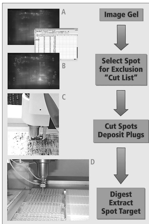
Figure 1. A schematic of the proteomics process from gel imaging to peptide processing. The image is a SYPRO Ruby-stain 2-DE gel (A). The spreadsheet inset shows the list of spots selected in a focused region of the gel (B). A self-washing tool cuts a gel for transfer to a microtiter well (C). The same tool uses a micropipette tip to dispense reagent into the processing wells (D).
